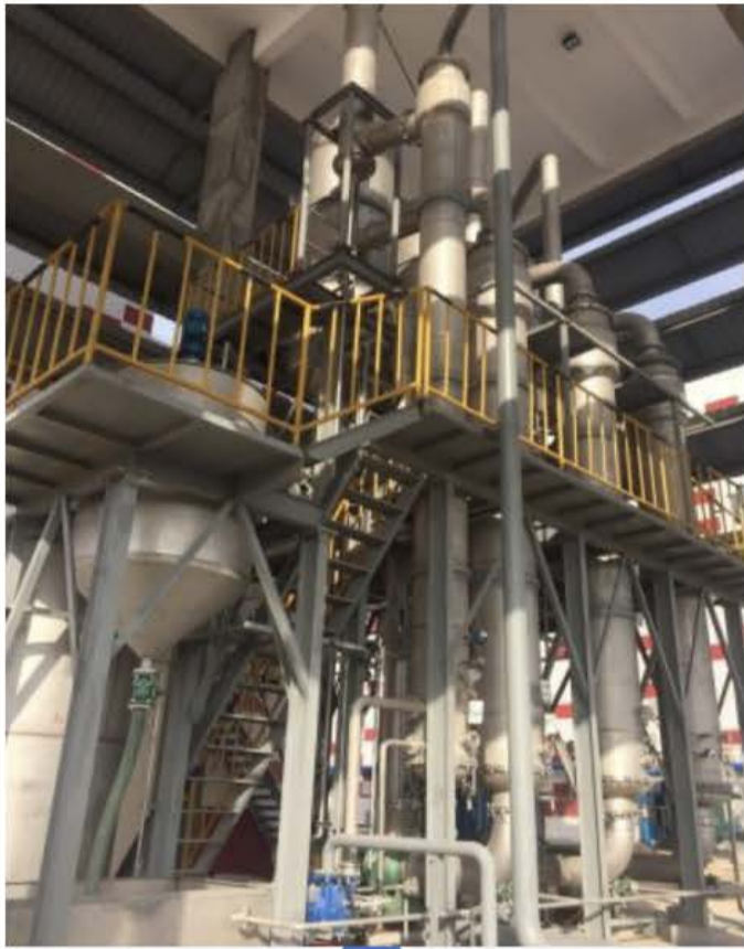
Triple-effect FC Evaporator ( Cobaltous sulfate )
