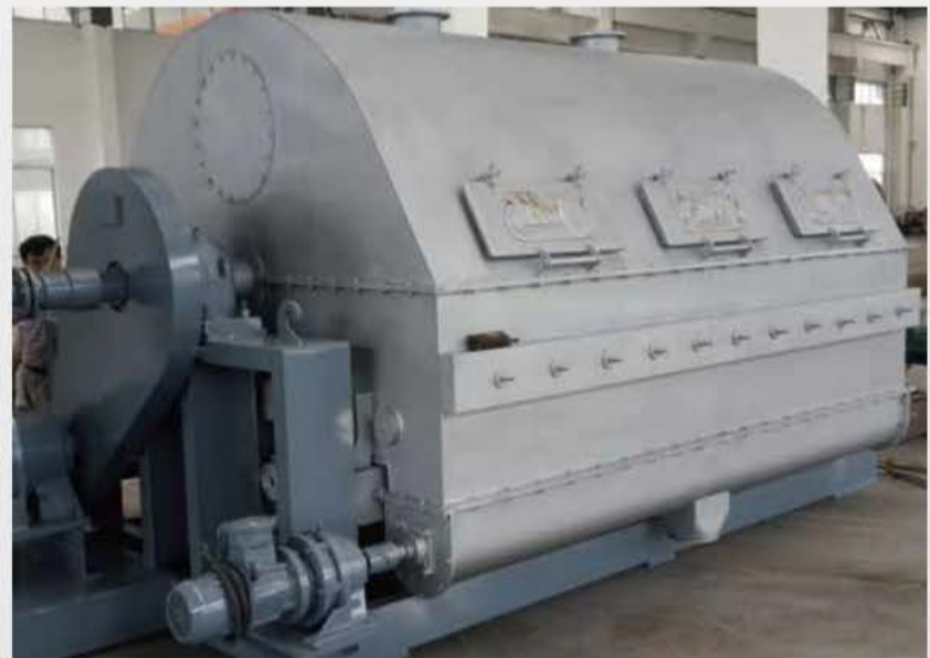
Enclosed type rotary drum flaker complete with screw conveyor
