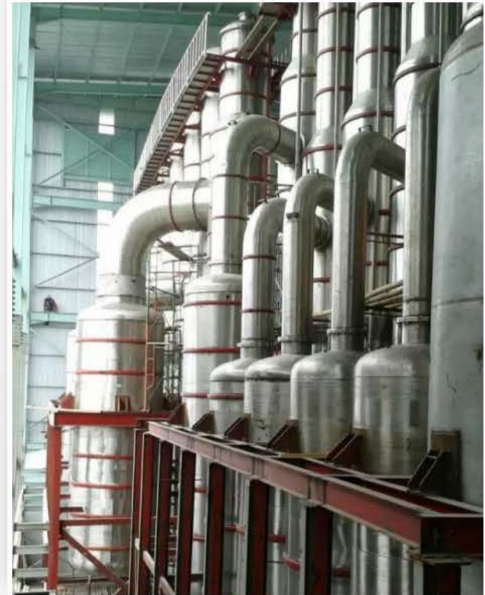
Five-effect FM Evaporator ( Glucose concentration )
