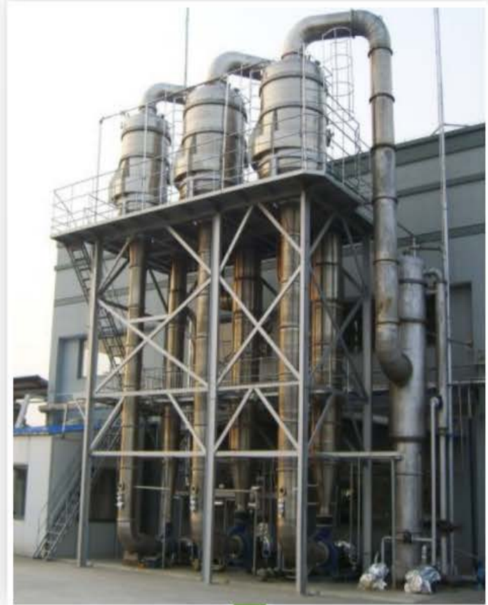
Triple-effect FC Evaporator ( Ammonium Chloride )
