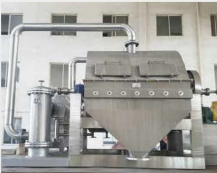
Enclosed type rotary drum flaker
