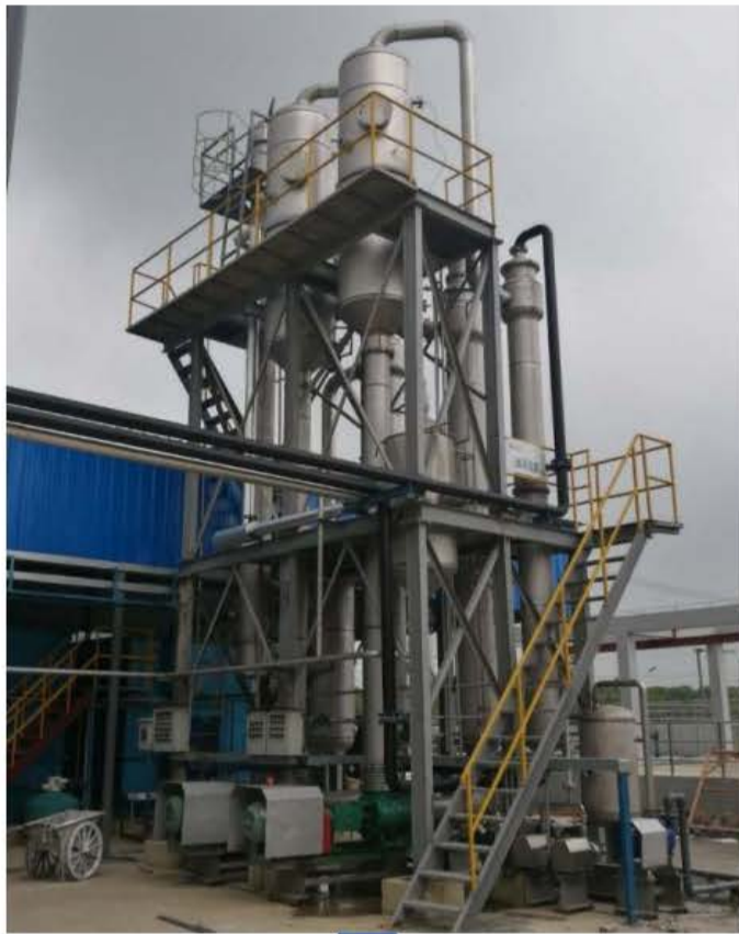
Triple-effect FC Evaporator ( Wastewater Treatment )
