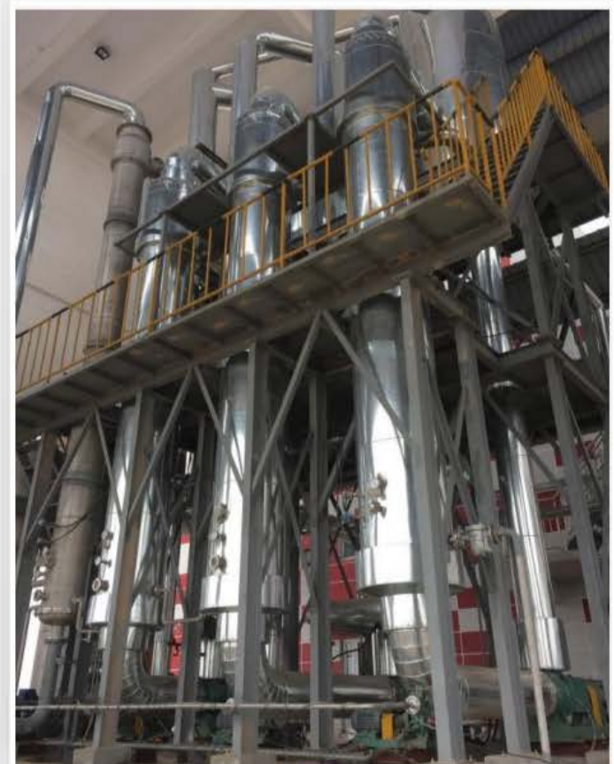
Triple-effect Evaporator ( Calcium lactate )
